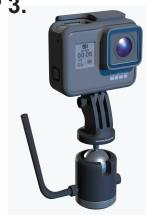
Aim the camera, and tighten both set screws to a snug fit. Tighten the socket cap screw in the 3-finger fork to secure the camera. Screws must be snug. Overtightening the screws will strip the threads.
